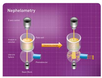
Nephelometry: scattered light is detected at incident angles of up to 80 degrees.
