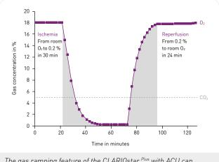
The gas ramping feature of the CLARIOstar Plus with ACU can mimic ischaemia/reperfusion conditions in vitro.
