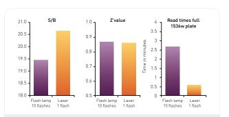
Comparison of xenon lamp (10 flashes; FL10) and TRF laser (1 flash; Laser1) for Signal-to-Blank (S/B), Z' value and read times.
