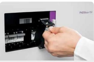
Our barcode-labelled Optic Modules are installed in seconds and automatically recognized by the reader.
