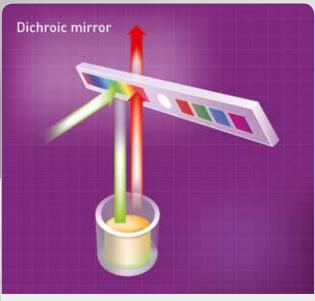
The Linear Variable Dichroic Mirror slide separates excitation and emission light further reduce undesired wavelengths.
