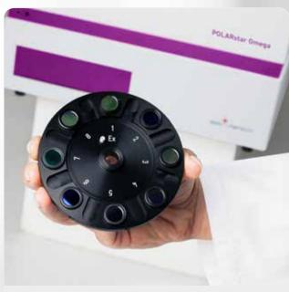
On the Omega series, a filter wheel can hold up to 8 different filters.
