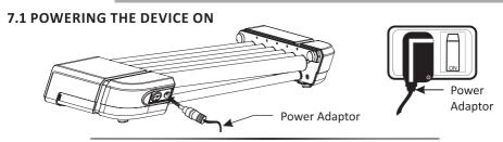
After connecting the power adaptor to back side of the device, switch the main power supply to "ON" & then switch the device on from the rear side. Make sure that tubes are loaded properly before use. Do not start the device if the hinge is open.
