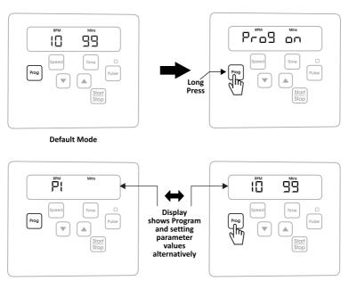
Press the "Program" button to select any program from "P1 to P9". Programs can also be selected by pressing "increment or decrement" button. Once the desired program is selected, press the "speed button" to select and set speed value. Press "Time" to select and set time value.
