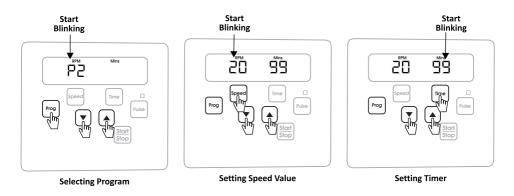
Speed and time value for that particular program is now saved. Press the "Start Button" to start the program mode operation. Once set RPM is reached, the program "Px" (with x = 1 to 9) and its "Speed" & "Time" value will display alternatively.
